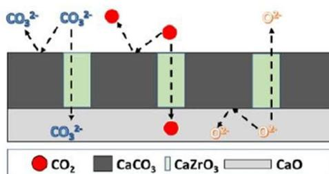
Graphical abstract: Facilitating the carbonation reaction of Limestone waste by using  $\text{CaZrO}_3$  nanoadditives.
