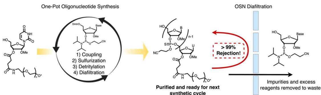
Figure 3: Schematic representation of OP-LPOS with OSN intermediate purification
